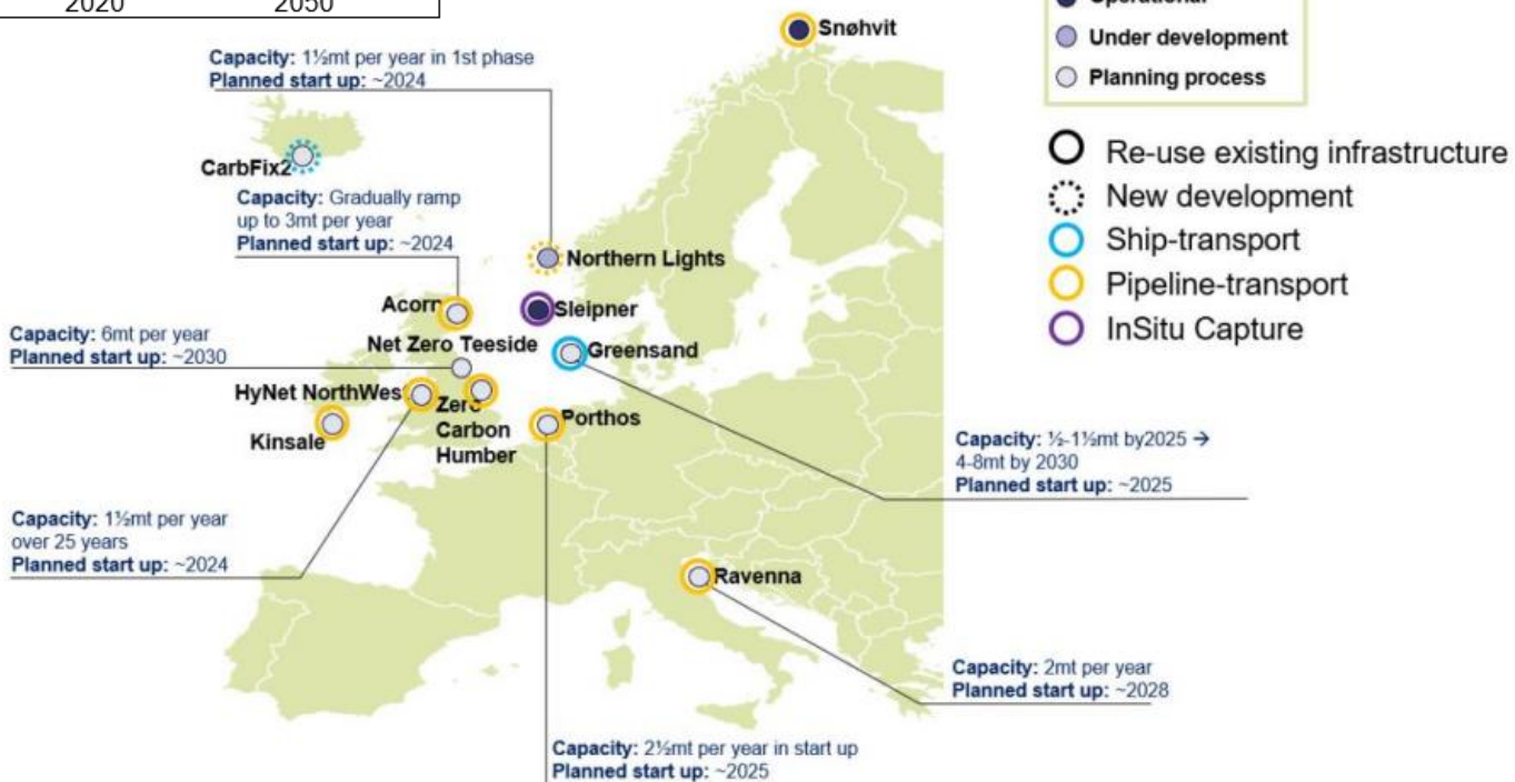
Figure 9: Overview of the operational, developing and planned CO 2 storage projects in Europe.
